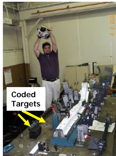
Figure 3. Measuring a Stamping Rail Panel Using Targets
